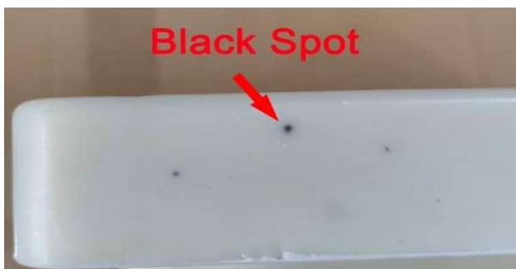
Gambar 2. Black Spot (Sumber : Topworks Plastic Mold)
